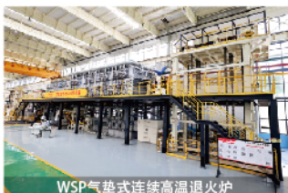
WSP AIR CUSHION CONTINUOUS HIGH TEMPERATURE ANNEALING FURNACE
